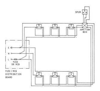
Fig 7.2.11.7.5: Arrangement of conductors in ring circuit connection
